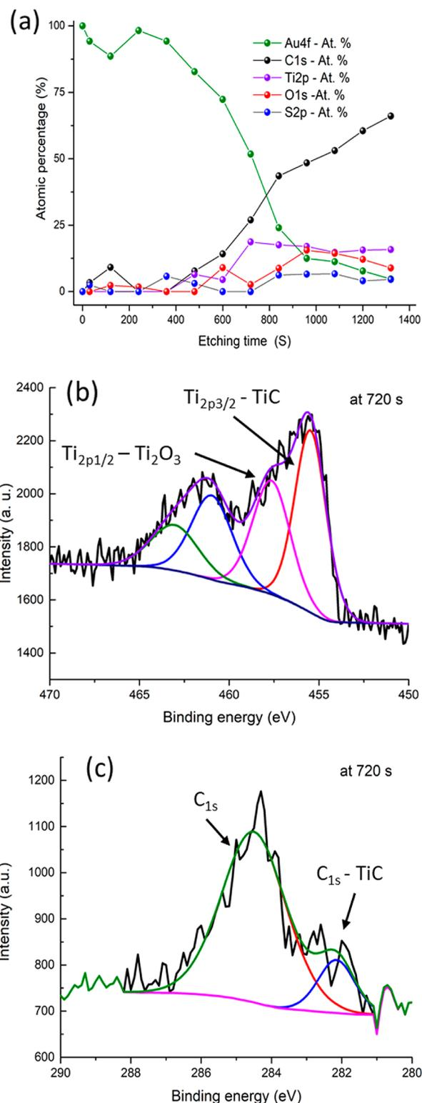
**Figure 3.** (a) Atomic percentages (%) vs etching time (s) for a Si/SiO<sub>2</sub>/PPF/BTB<sub>9</sub>/Ti<sub>2</sub>/Au<sub>20</sub> (b) titanium high resolution XPS signal, (c) carbon high resolution XPS signal.
